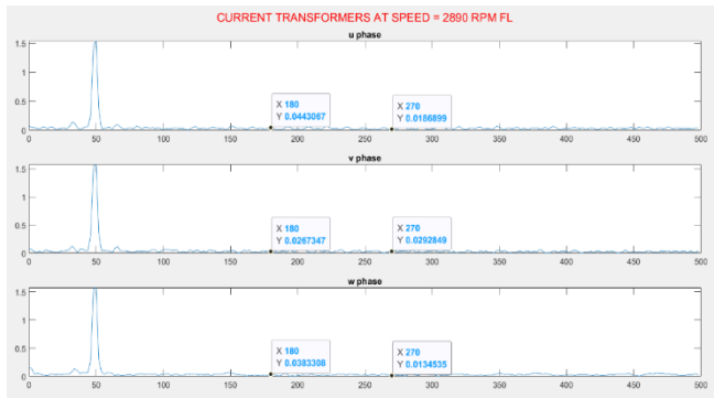
Fig. 11. Fault analysis for bearing failures using current transformers readings
