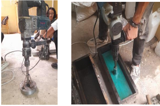
Figure 1. Vibrator Compaction Hammer
